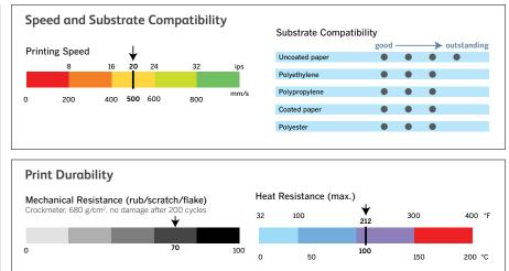
Videojet evaluation of observed performances of the Regular Grade Ribbon with optimized printer setting and receptors
